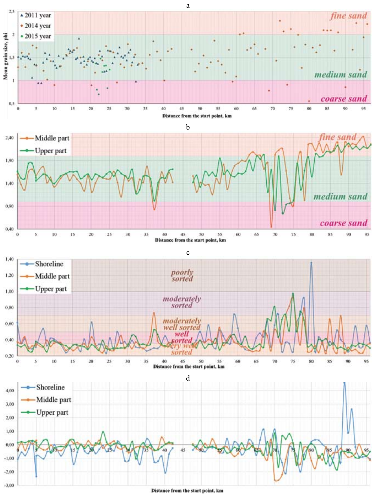
Fig. 3 Alongshore variations of grain size characteristics for the samples collected along the Curonian Spit shore: mean size (in \phi units) for (a) shoreline (all three years 2011, 2014 and 2015) and (b) beach sediments (middle and upper parts, 2014), (c) sorting (2014), and (d) skewness (2014). Compiled by O. Kovaleva, 2015
